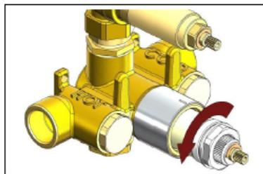
3. Remove the thermostatic cartridge and clean its filters under running water or leave to soak in vinegar in presence of limescale. Grease the O-rings and, if damaged, replace them with new ones.
