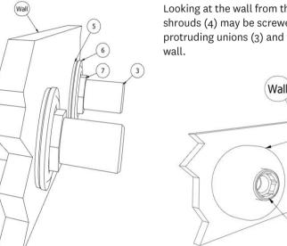
Looking at the wall from the front, the wall shrouds (4) may be screwed over the protruding unions (3) and fixed tight up to the
