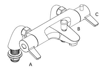
When the diverter (B) is in the lower position, water will flow through the bath filler spout. To divert water through the hose to the shower head, raise the diverter handle to be in the raised position. The diverter will remain raised until manually lowered.
