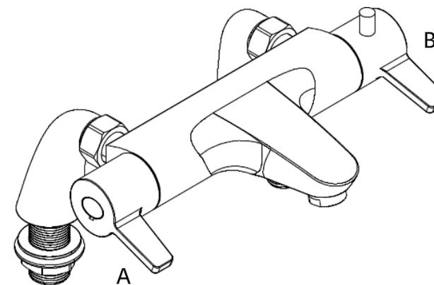
Handle (A) controls the flow. Raise the handle to increase the flow of water from the bath spout.
